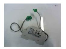
Unscrew 4 torxscrews in de ForcelQ control box and put the control board upside down
