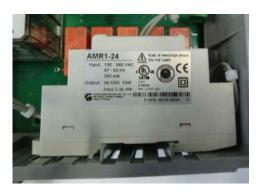
Snap the power supply onto the plastic rail of the circuitboard housing
